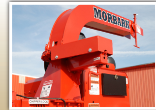
DISCHARGE 360° Manual Crank Swivel Discharge
