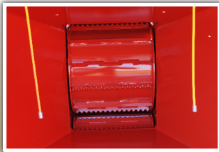
TOP FEED WHEEL 18" diameter top feed wheel with combination serrated teeth and knife bars
