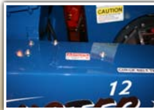
DRIVE BELT COVER Drive belt inspection cover provides ease of drive system maintenance
