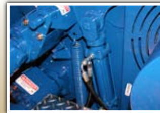
HYDRA-LIFT SYSTEM Hydra-Lift Compression System with spring assisted down pressure
